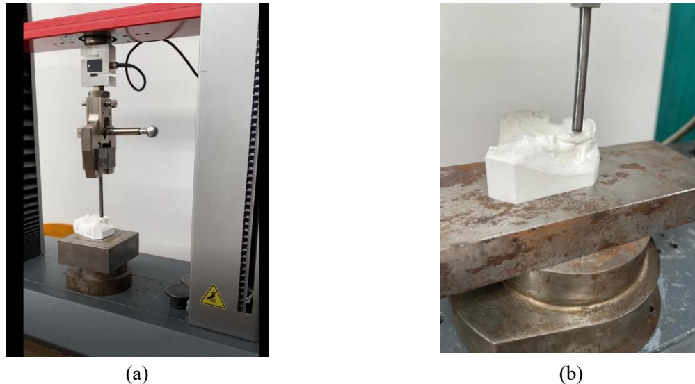
Figure 4. (a) Mechanical compression testing performed using the Zwick/Roell Z005 universal testing machine. (b) Detailed view of the experimental setup, showing the positioning of the space maintainer on the supporting model and the application of axial load through the loading rod during the compression test.
